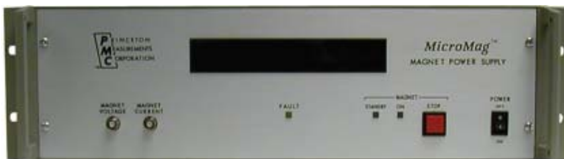
図 18 Magnet Power Supply(front view)
